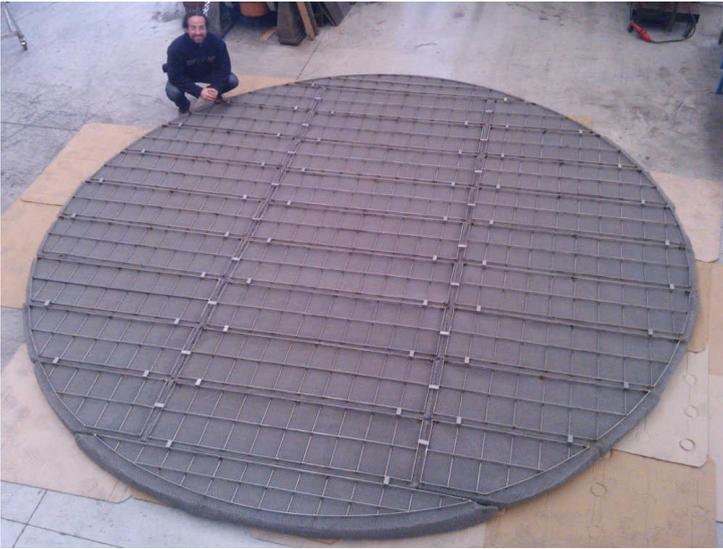
Wire mesh separators are widely used when an effective separation between liquid and aeriform phase is very important in order to obtain cheap and efficient industrial processes.
