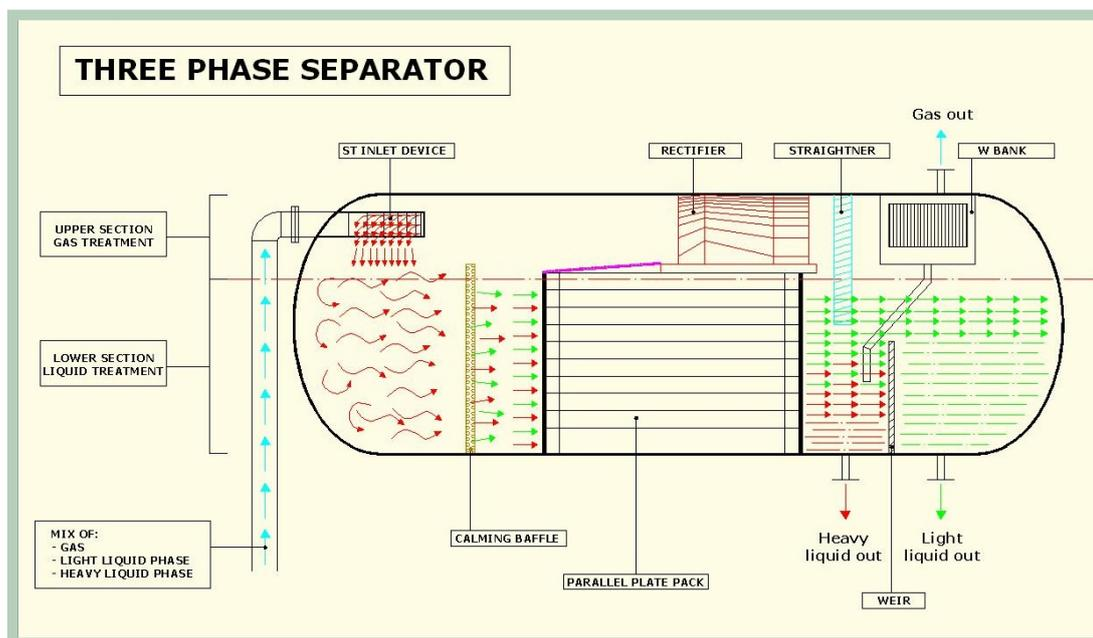
**Process:** in general a ST inlet separator is used to calm and distribute the flow at the entrance of the vessel and, to obtain the separation of the three phases, the flows are forced to pass through some internals at the same time but in two different sections of the vessel:
