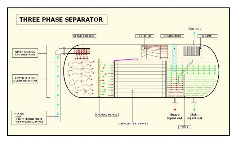
**PROCESS:** In general a ST inlet separator is used to calm and distribute the flow at the entrance of the vessel and, to obtain the separation of the three phases, the flows are forced to pass through some internals at the same time but in two different sections of the vessel:
