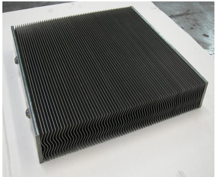
This kind of special vane pack is often used in "steam drums" located over cyclones to eliminate small liquid droplets drained by vapour stream.
