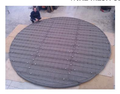
Wire mesh separators are widely used when a effective separation between liquid and aeriform phase is very important in order to obtain cheap and efficient industrial processes.
