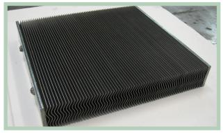
The so called "W bank" is a particular kind of vane pack used when to shorten the length of the tank is a priority. Thanks to its paritcular "V" shape it's possible, with half lenght of the pack, to obtain an equivalent crossing area and to reduce the dimension of the vessel.
