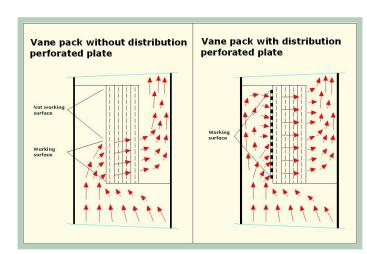
The problem can be solved applying a perforated distribution sheet that forces the distribution of the flow all over the available area of the vane pack window (see the scheme below).
